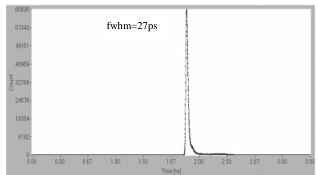
Fig 5: System response for the R3809U-50 MCP
