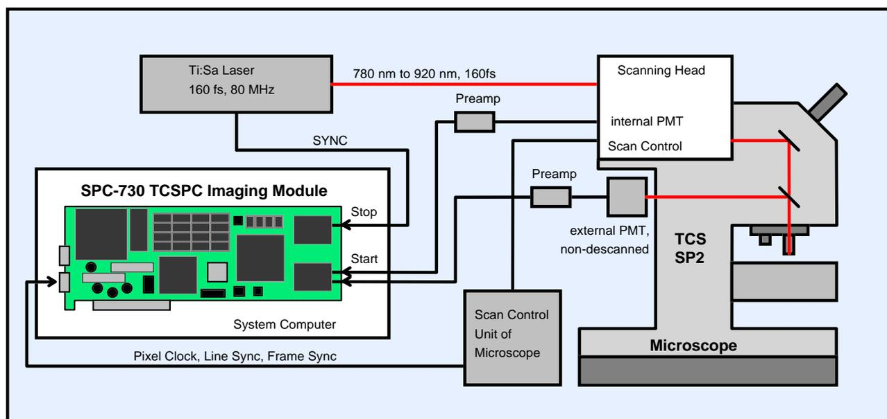
Fig. 2: Basic setup of the TCSPC Laser Scanning Microscope
