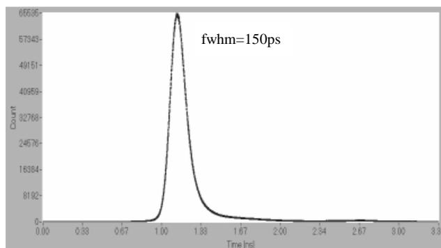
Fig 4: System response for the PMH-100 detector
