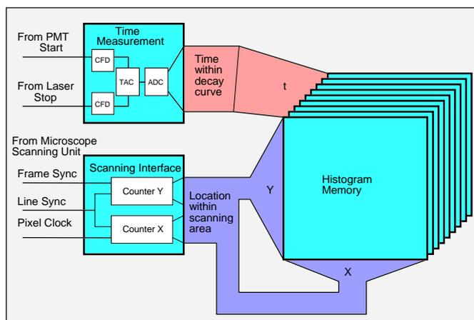
Fig. 2: Basic principle of the SPC-730 TCSPC Imaging module
