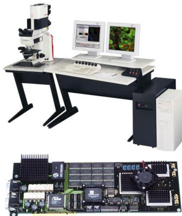
Fig. 1: The Leica SP-2 Laser Scanning Microscope and the Becker & Hickl SPC-730 TCSPC Imaging Module
