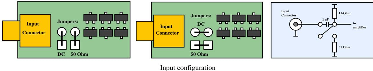
When the jumpers are inserted the configuration is 'DC' and '50  $\Omega$ '. To change the configuration to 'AC' or '1k  $\Omega$ ', pull off the corresponding jumper.
