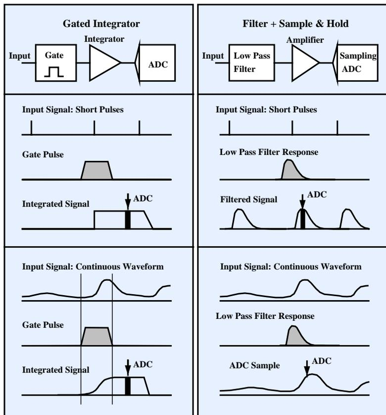
Comparison of the Gated Integrator and the Filter + Sample & Hold architecture of the SHM
