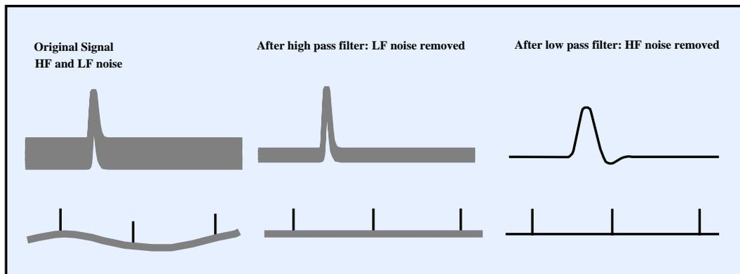
Effect of filtering on signal-to-noise ratio
