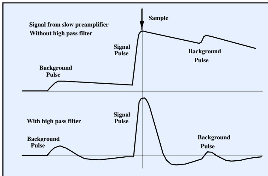
PMT signal from slow preamplifier. The high pass filter helps to unmix background and signal pulses
