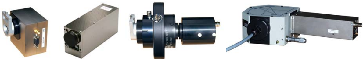
Fig. 3: Left: bh PMC-100 detector module, with RLD adapter. Second left: HPM-100-40 hybrid detector module. Second right: R3809U MCP PMT, with shutter and RLD adapter. Right: bh MW FLIM multi-spectral detection assembly
