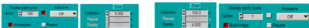
Fig. 6: Parameter definitions for online display. Left: Scan Sync In mode. Right: FIFO Imaging mode.
