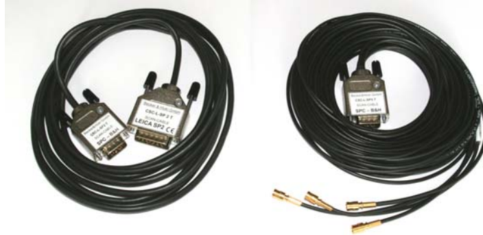
Fig. 5: Scan control cables of the Leica NDD FLIM systems. Left: SP2. Right: SP5. The cables are the only electrical signal connection between the microscope and the FLIM system.
