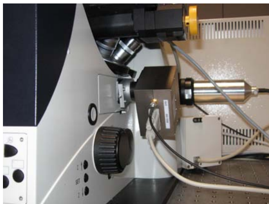
Fig. 4: PMC-100 detector attached to the RLD port of a Leica SP5 multiphoton microscope
