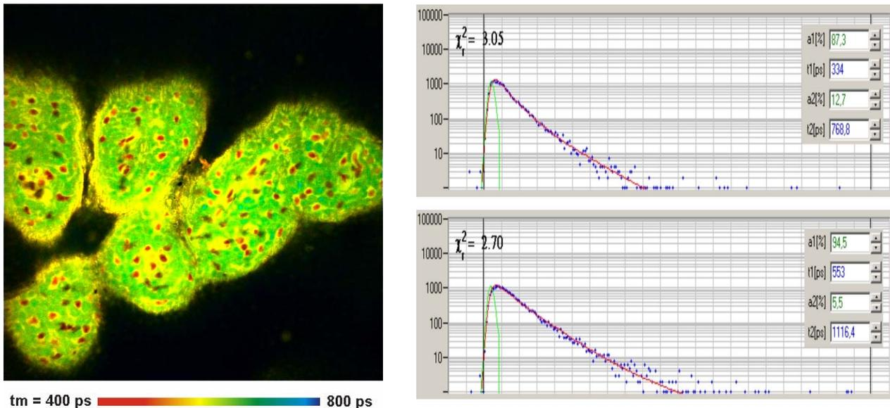
Fig. 3: Pig skin stained with methylen blue. Left: Lifetime image, double-exponential model, amplitude-weighted lifetime. Right: Decay curves in 3x3 pixel areas. Top: From red spots (fast decay). Bottom: From green areas (slow decay)
