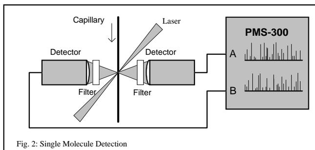
Fig. 2: Single Molecule Detection
