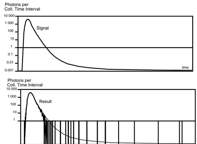
Fig. 5: Recording a wide dynamic range signal in the Event Mode
