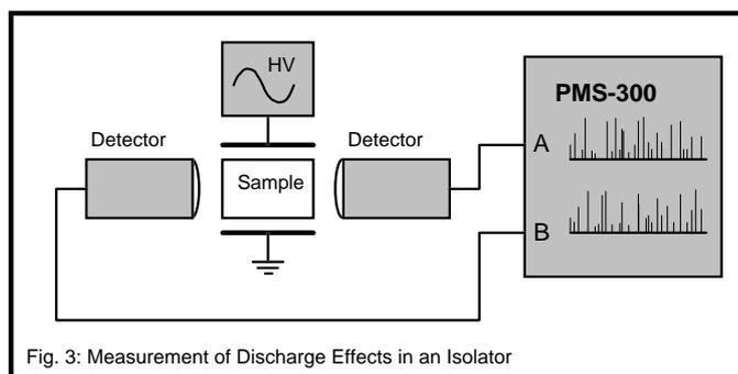
Fig. 3: Measurement of Discharge Effects in an Isolator
