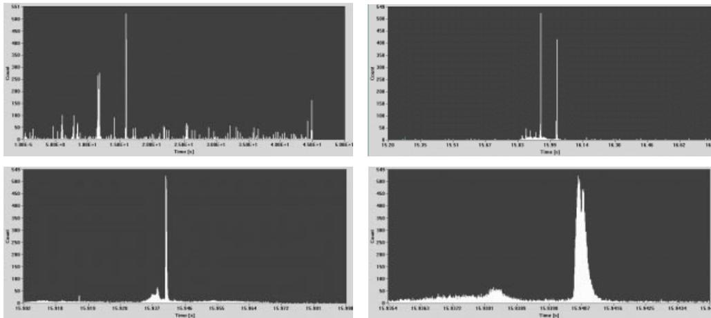
Fig. 7: Lightning bolts in a thunderstorm. Collection Time 10 us, Event Threshold 4 counts.
